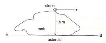
Estimate the horizontal distance from the stone's point of projection along the line AB at which the stone lands. Ignore the curvature of the asteroid.
