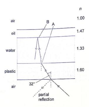
The light is refracted at an angle of 32° when it enters the plastic layer as shown.
